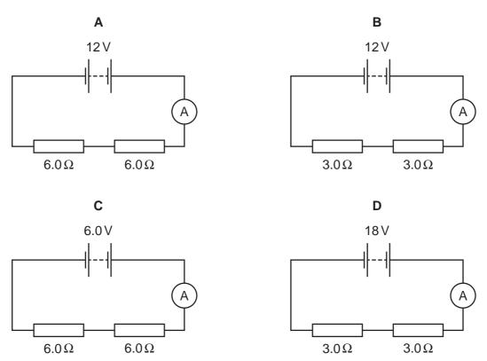
33 In which circuit does the ammeter read 2.0 A?
